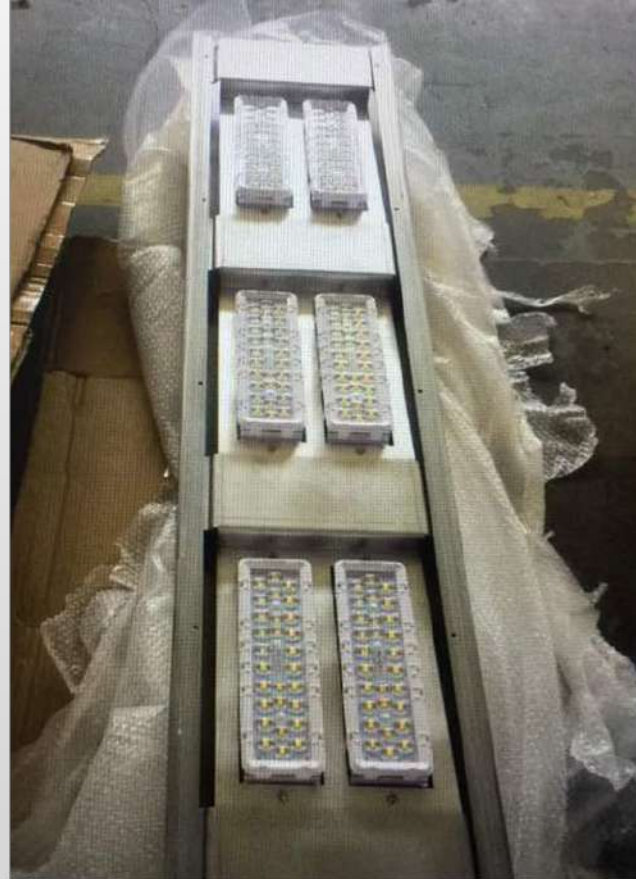
Developing IP68 LED light modules using Cree Diodes and MSI Heatsink lens and housing, and integrating into Pole Light Arm
