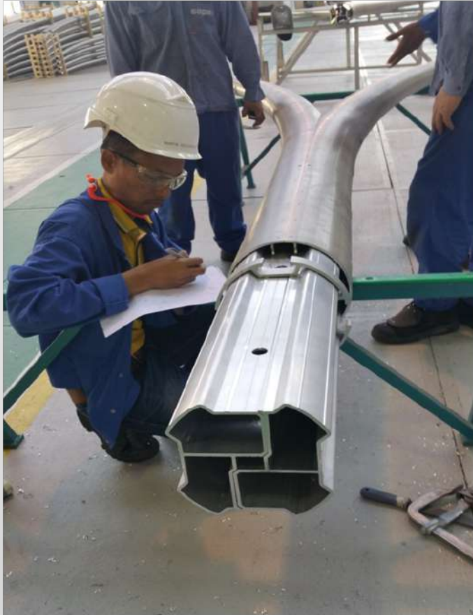
Developing new twin arm 12m decorative multifunctional pole
