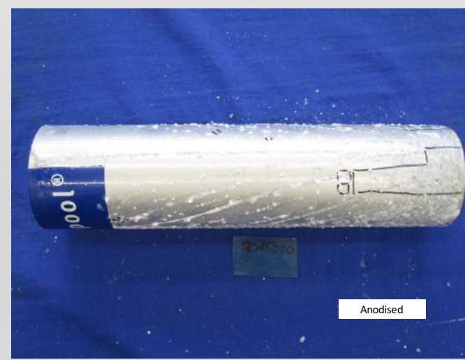
1,000 Hour Salt Fog Test Samples for Education City & Oman Sea Wall – Batinah Hwy
